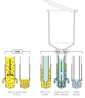
1,000-fold buffer exchange in a single spin. Protein (purple dots) is dissolved in Buffer 1 (yellow) during the concentration step (left). During the buffer exchange step, 1.5 mL of Buffer 2 (blue) is added. Arrows indicate direction of fluid flow, showing that Buffer 2 enters the sample continuously while Buffer 1-containing solution is being forced out.
